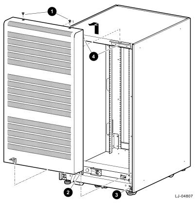
Figure 2-4 Removing and Replacing the Rear Lift-Off Door
